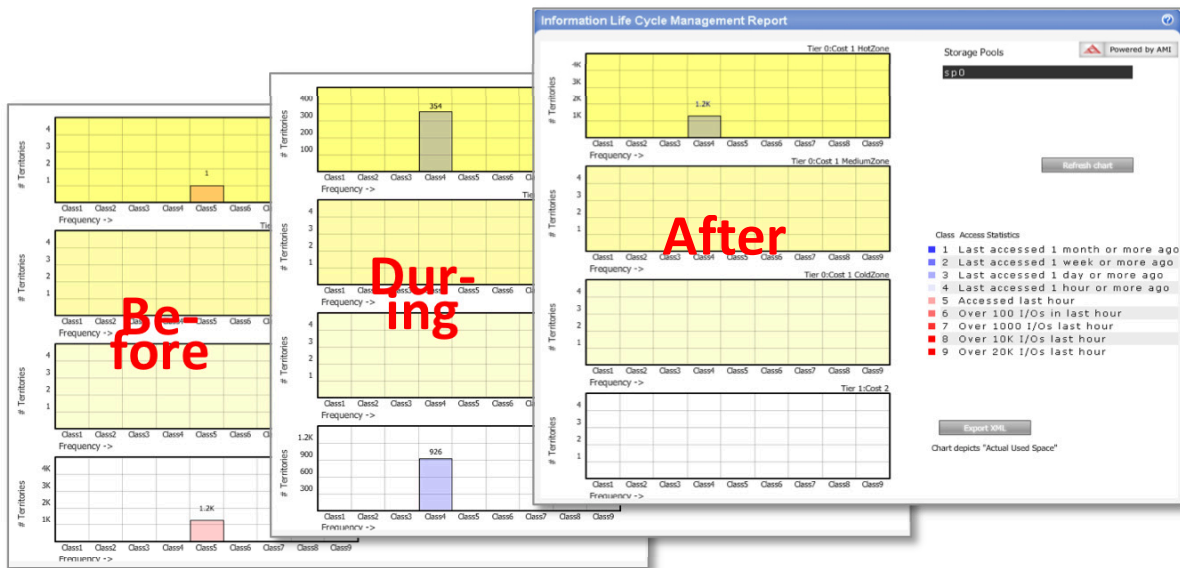
Figure 11: StorTrends 3400i ILM interface shows the auto-tiering of data across storage types and on the individual spindles themselves (each SAS disk is divided into three zones within Tier 0 above, to help optimize the access time and throughput for critical data). At the beginning of our test, 1.2K 1MB blocks underlying our test volume were stored on SATA disk (Tier1). By the end of our test all 1.2K 1MB blocks were on Tier 0.
